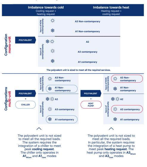
In the case of **multi-unit** configurations, the coupling of the two units can be easily managed via the MTM management system, which allows efficient decision-making on the start-up and operating strategies of the units.
